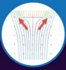
As ink is a liquid it will flow around any obstacle i.e. A closed ink key, subsequently disrupting any adjacent keys flow. This means every key or sweep adjustment will affect flow characteristics & impact presets.
